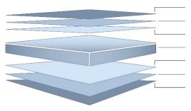
Finish Coat (Finish Coat + Primer = nominal 25µm) {Refer Notes 4 & 5} **Corrosion Inhibitive Primer Conversion Coating** Grade 430 Stainless Steel **Conversion Coating Corrosion Inhibitive Primer** Backing Coat (Backing Coat + Primer = nominal 10µm total) {Refer Note 6}
